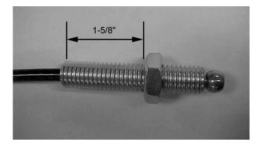
Figure 7. Thread the nut onto the cable.
